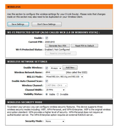
**Enable Auto Channel** The **Auto Channel Scan** setting can be selected to allow the DIR-632 to choose the channel with the least amount of interference.
